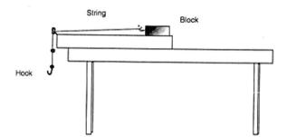
Practice pulling the block along the board by putting washers on the hook. *The back end of the block should cross the starting line.* The number of washers on the hook is a measure of the amount of **force** needed to pull the small block forward.
