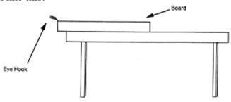
Put the small **block** on the board. Place it <u>behind</u> the red starting line. Take the string with the big metal hook and pull it through the small eye hook. Now loop the string onto the hook on the block. It should look like this:
