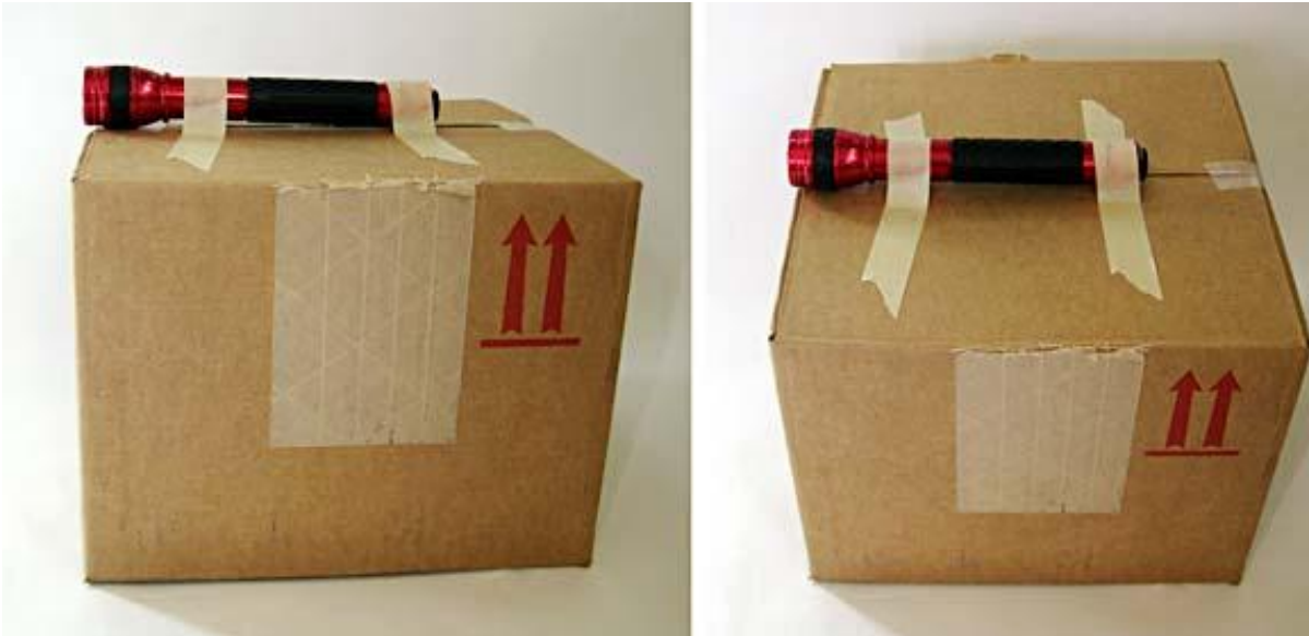
Figure 3. Place the cardboard box, stepping stool, brick, or block of wood on a firm surface and tape the flashlight to the top so that the flashlight's edge is close to the box's edge.
