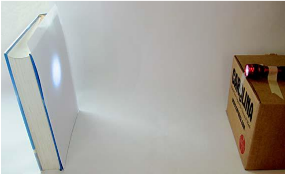
Figure 6. Move the graph paper further from, or closer to, the flashlight until a crisp, 5 - 6 cm diameter circle of light forms on the graph paper.
